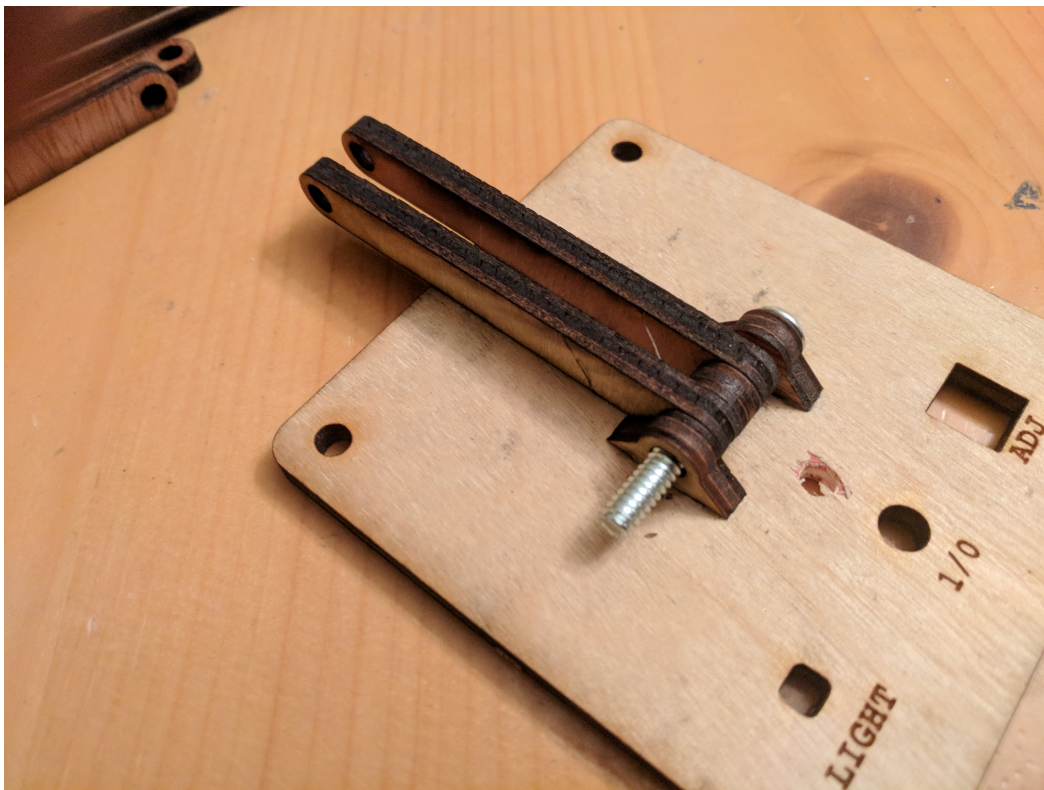
Figure 5: 10-24 bolt through the pivot joint on the base, add a spacer between the first two arm pieces
