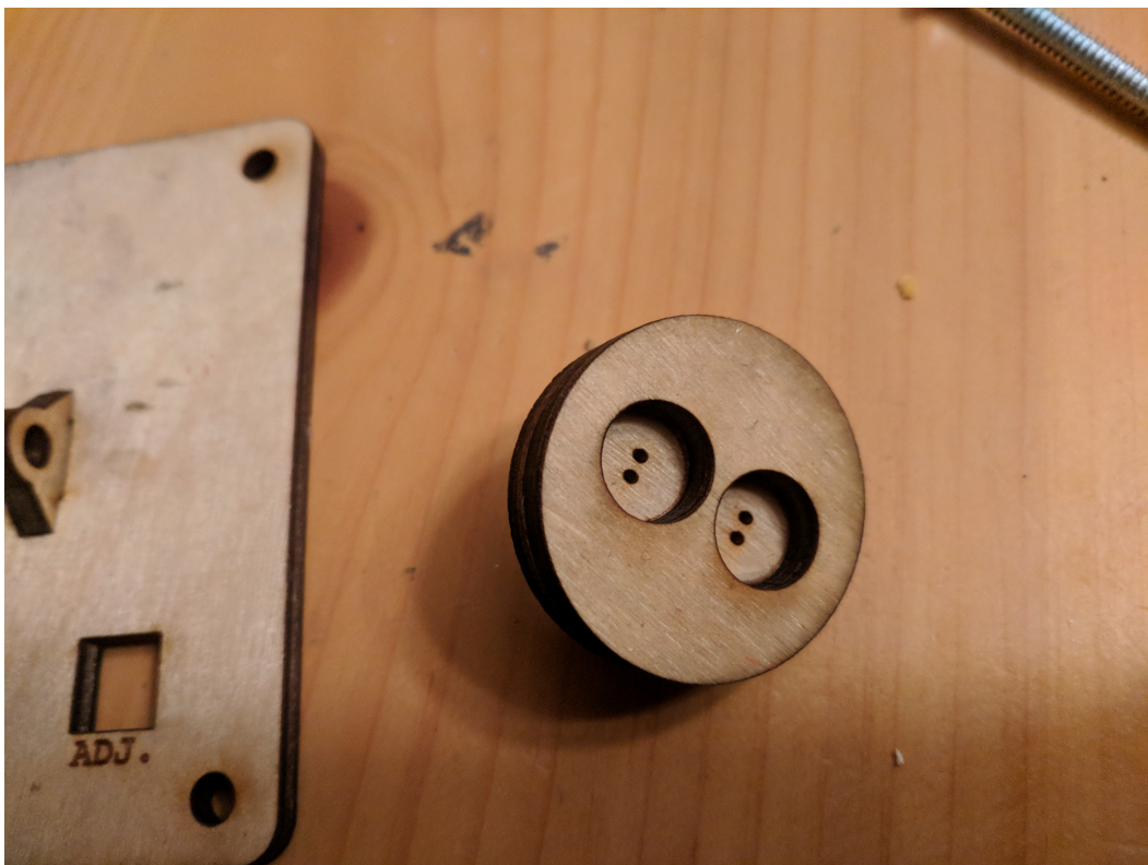
Figure 4: Align and glue the two lamp head pieces together
