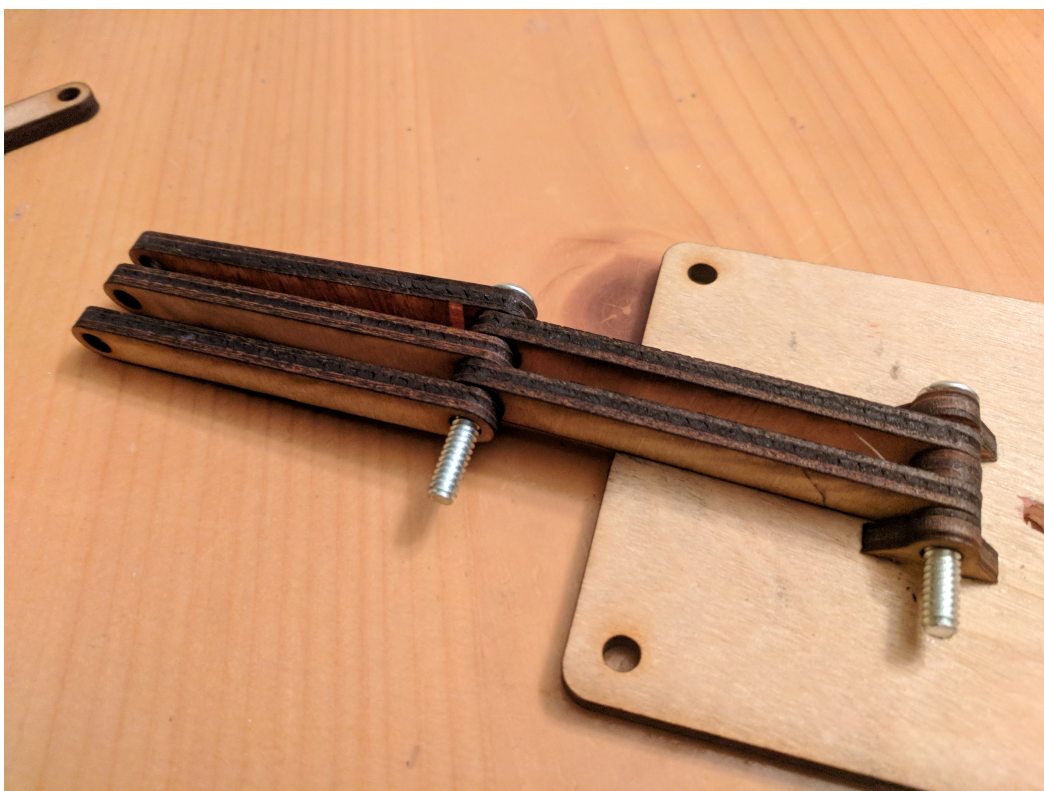
Figure 6: Add three more arm pieces and place a 10-24 bolt through those 5 stacked
